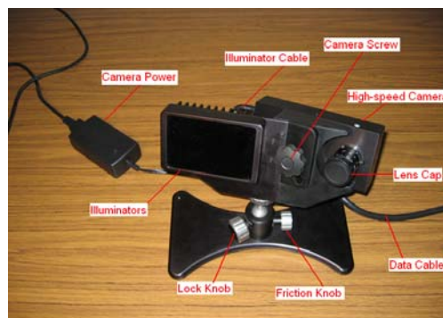
Figure 3-5: Parts of the EyeLink 1000 Desktop Mount
